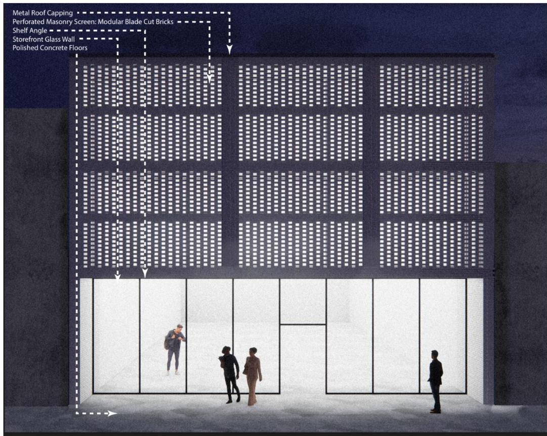
As a group, we wanted to do a masonry façade that was not necessarily solid. We wanted to be able to manipulate the space more than a solid face with punched windows. Because of this, we landed on the idea of a having a screenlike façade that allowed light to filter through into the spaces behind.
